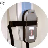
The Chamber Adapter makes it possible to use Ion Chambers with the Piranha. It is primarily designed for Mammography and CT use, but can of course be used for other applications as well.
